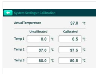
Accurate temperature control with 3-point calibration
